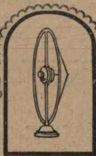
A cone diaphragm loud speaker can easily be constructed. The illustration shows one method of mounting.
